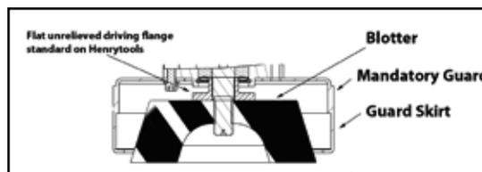
Cup wheels are mounted directly onto the tool. No additional accessories are required.
